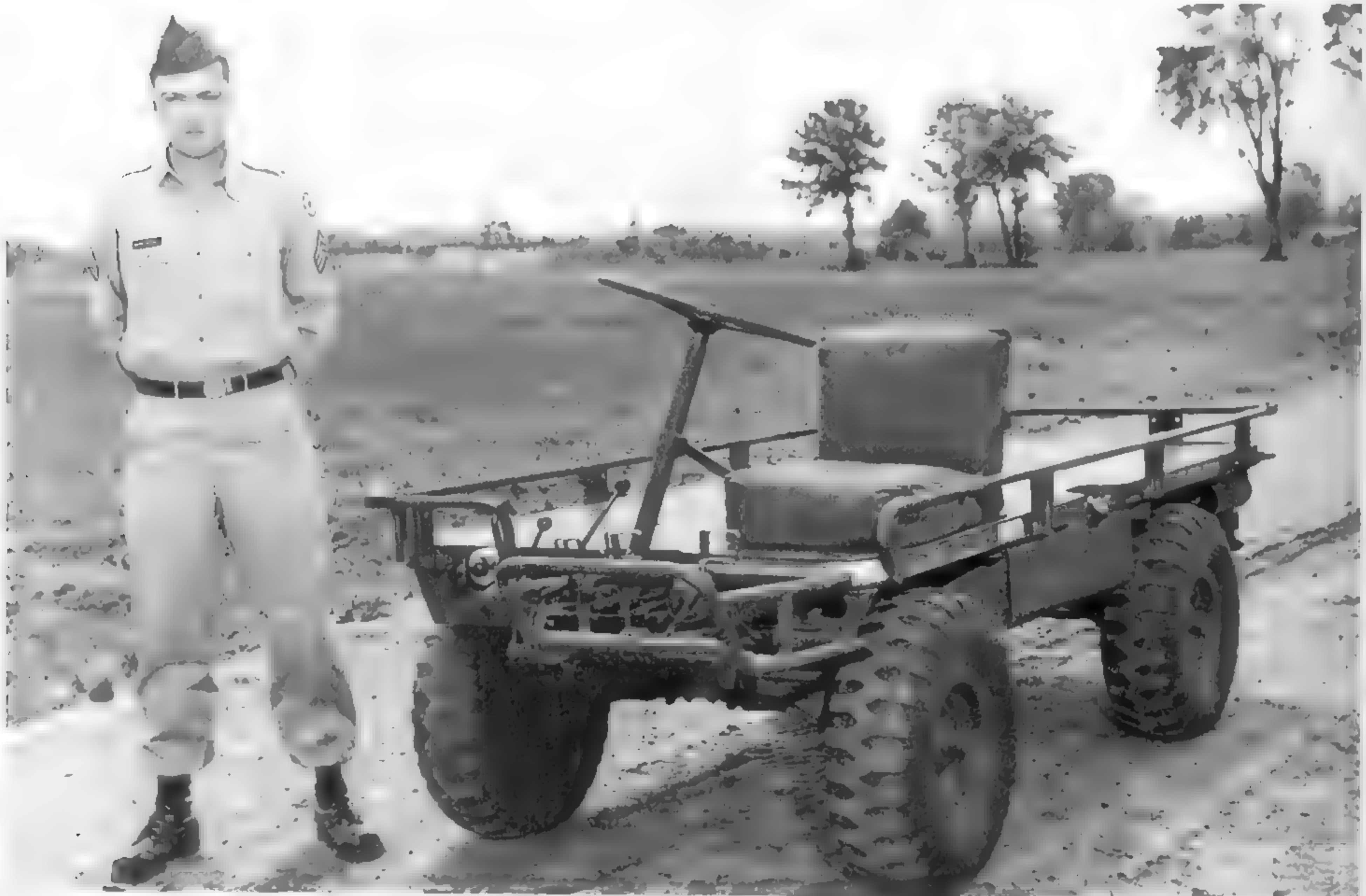
The height of the steering column in the Mule made it within easy reach of a soldier walking. It could be swung forward and driven in reverse in that manner, allowing the driver's seat to be stowed and cargo placed in its position. (U.S. Army photo)
